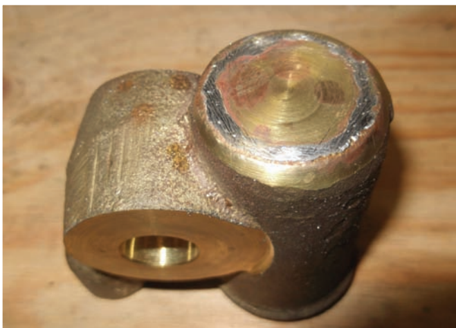
Bottom of Trunnion After soldering
