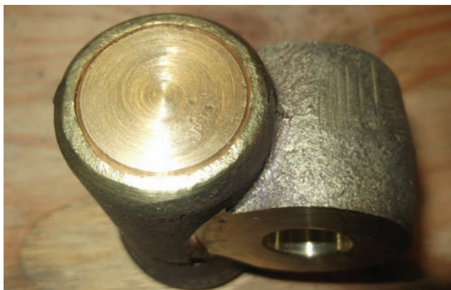
Bottom of Trunnion showing blanking disc
